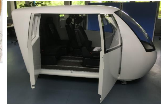
Cabin design and hardware for mixed-reality passenger acceptance studies
