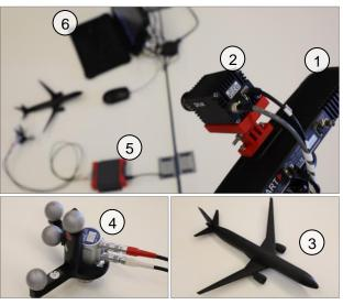
FIG 4. Setup of the hybrid tracking system
