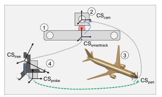
FIG 6. Illustrated transformations in the Hybrid Tracking System for NDT
