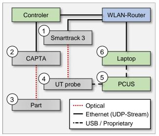
FIG 3. Structure of the hardware setup
