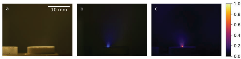
Figure 15: Gypsum sample on the sample stage inside the vacuum chamber before and during LIBS measurements. a) Image before LIBS measurement. b) Laser-induced plasma plume during LIBS measurement. c) False-color image of emission captured with a 656.3 nm bandpass filter.
