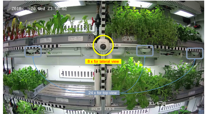
Fig. 3: Camera layout scheme example. Blue - top-view cameras; yellow - lateral cameras.
