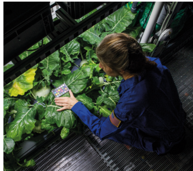
Prof. Dr. Anna-Lisa Paul (University of Florida) calibrating the multi-wave length sensors with a dedicated color plate; Source: Esther Horvath (AWI)
