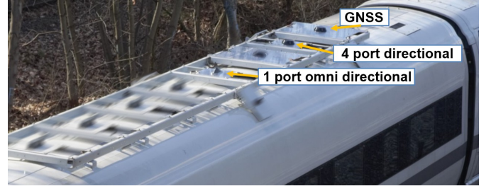
Fig. 2. Antennas installed on DB Advanced Trainlab
