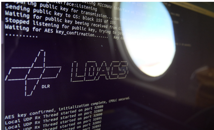
Figure 1.17: Console output during after successful key exchange. All further communication afterwards was secured using AES-256-GCM.
