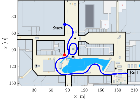
Figure 4: The indoor simulation scenario with one physical transmitter indicated by the red triangle labeled Tx and the reference track depicted by the blue line. Black lines indicate walls that reflect the transmit signal, and black dots represent point scatterers such as pillars.
