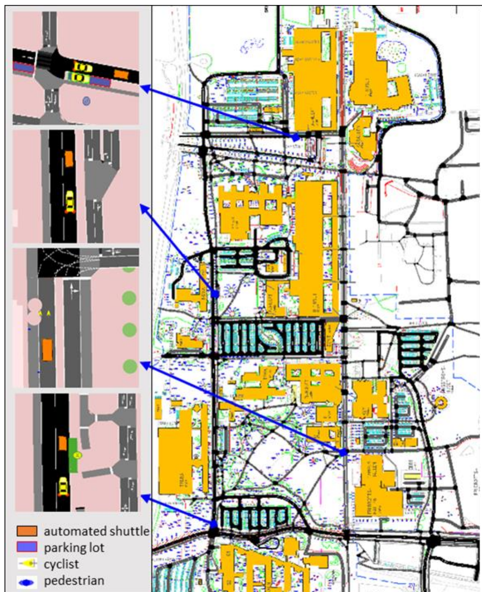
Figure 9 Simulation network built with SUMO (background map source: Akademiska Hus)
