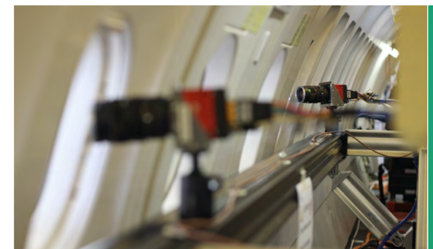
A stereo camera system installed in the aircraft cabin was used to measure the deformation of the wing during various flight-test manoeuvres
