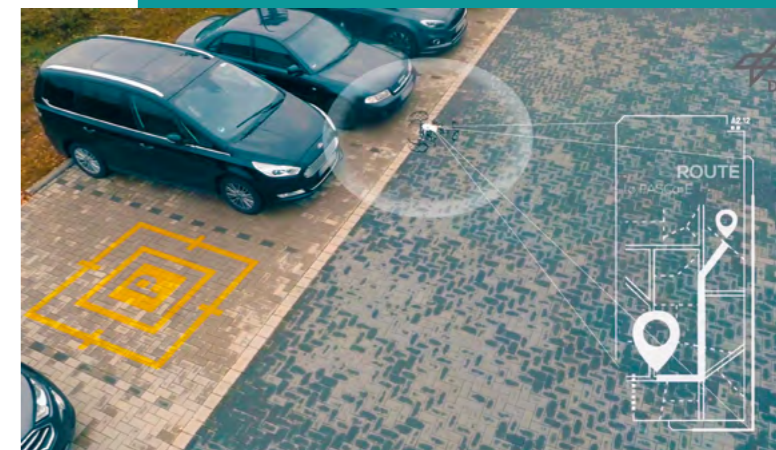
DLR tested autonomous parking in the AUTOPILOT project. Using an App, the driver sends the car to search for a parking space. With the help of a drone, the system identifies a suitable spot, navigates the vehicle to it and parks.
