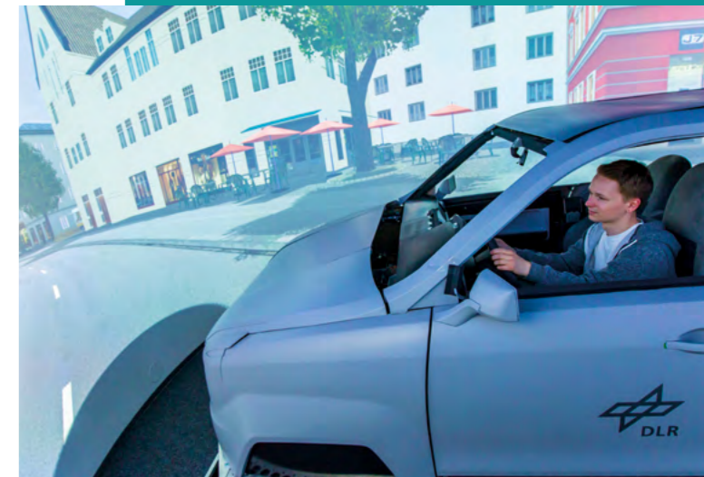
At its Virtual Reality Lab, DLR is conducting research into automated and networked driving. To ensure that tests are conducted under as realistic conditions as possible, there is room in the laboratory for a medium-sized car, and the 360-degree display provides a panoramic view.
