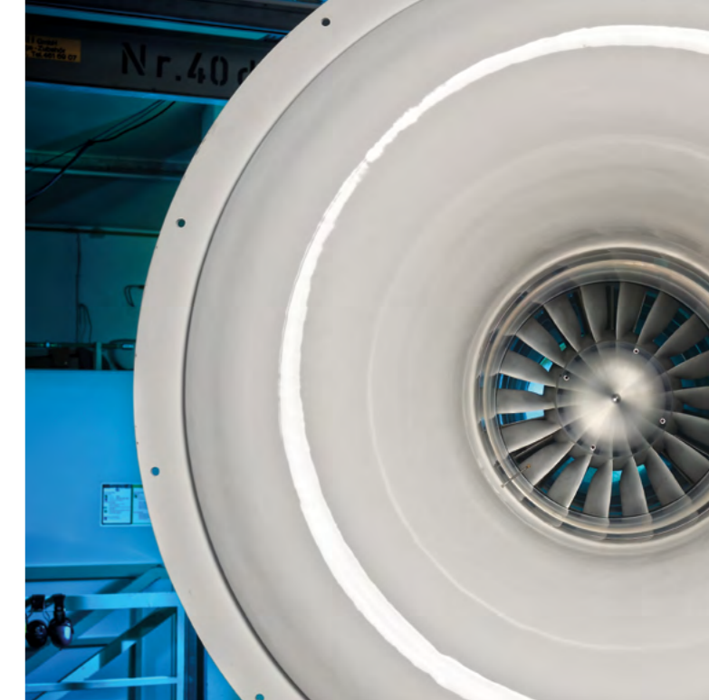
View into the inlet of the CRAFT test stand
