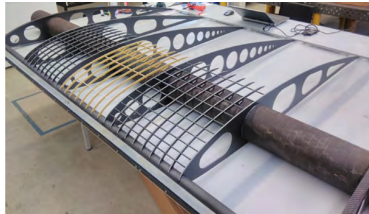
The wings of the platform consist of a sandwich rib structure made of carbon fibre reinforced polymers (CFRP). A round CFRP tube forms the backbone. This makes the wing light and stable. In total, the structure of the HAP alpha weighs 36 kilograms, 75 percent of which is the main wing.
