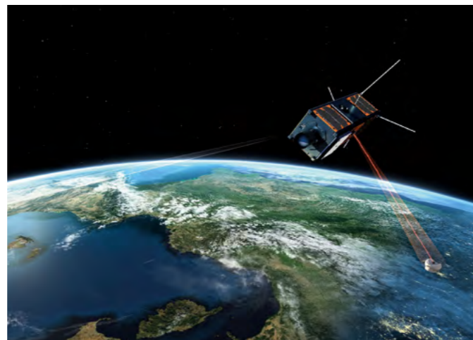
The PIXL-1 satellite carries the OSIRIS4CubeSat laser terminal, whose system consists of a highly compact combination of electronics, mechanics and optics.
