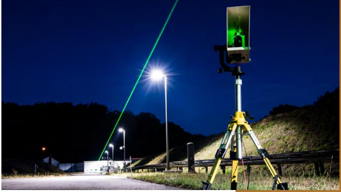
Since the opening of the Laser Test Range in 2008, a team of researchers at the Institute of Technical Physics has been investigating the properties and propagation of laser radiation under real atmospheric conditions. With the help of this facility, which is the only one of its kind in Europe, eye-safe laser systems and laser spectroscopy technologies are developed. One application is the detection of hazardous substances from a safe distance
