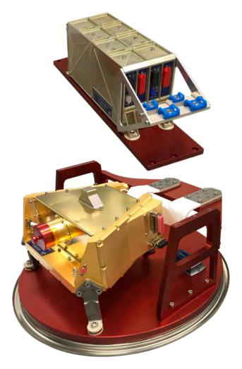
The CHEOPS focal plane module (bottom, base plate diameter about 40 centimetres). Above it is the module for the sensor control electronics. Both modules were developed and built at the DLR Institute for Optical Sensor Systems in Berlin-Adlershof.
