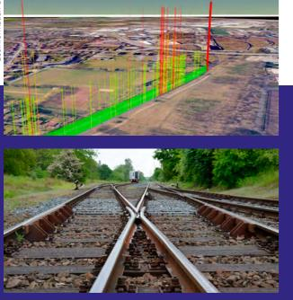
Condition monitoring systems can also be used to examine railway infrastructure, as depicted here with a shunting locomotive at Braunschweig harbour. Sensors in the vehicle's axle bearings continuously measure vibrations. This resulting data give information about the condition of the track.
