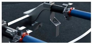
Visualisation of the crash absorber. In the event of a collision, the telescope-like tube (blue) in the front car is severed by an annular cutter (red) and thus absorbs a large part of the kinetic energy.
