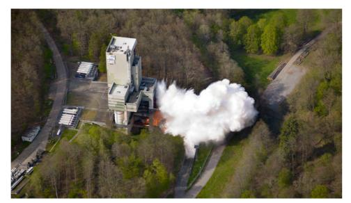
Every test on a main-stage engine is an impressive event. A Vulcain 2.1 consumes 600,000 litres of liquid forming pure water – during a firing duration of approximately 12 minutes. Together with the water used for cooling, this forms the characteristic steam cloud above the test site. Later, this falls back to Earth
