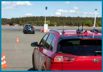
Special robotic cars driving on pre-programmed routes simulate the surrounding traffic
