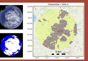
The original image from the cloud camera (above left) shows the whole sky above the measuring station, from horizon to horizon. These data only become meaningful once they are rectified and, as here, projected onto the Oldenburg urban area.
