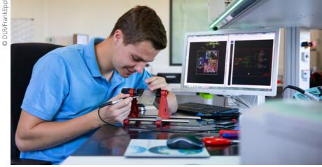
Fabian Staiger, a trainee system electronics engineer, soldering a circuit board.
