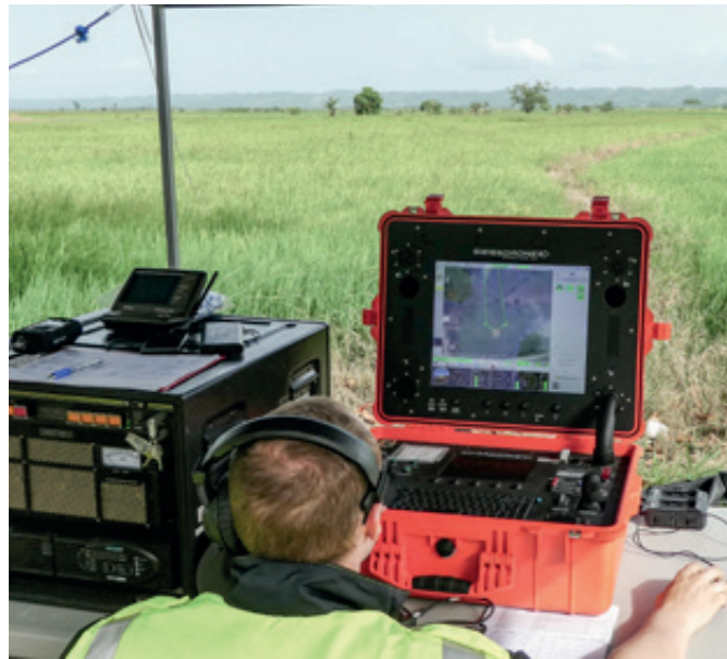
Humanitarian mission in the Dominican Republic: In July 2018, the DLR Institute of Flight Systems conducted flight tests to transport relief supplies to hard-to-reach areas with the unmanned helicopter superARTIS. The flights were planned and monitored from the mobile ground control station.
