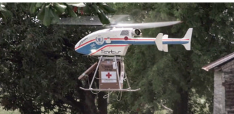
The small unmanned helicopter superARTIS (Autonomous Rotorcraft Testbed for Intelligent Systems) is operated as an experimental carrier by the DLR Institute of Flight Systems. Its range, robustness and payload capacity make it well suited for humanitarian missions.
