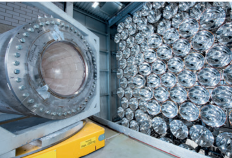
Thermal hydrogen production experiment using solar radiation from the Synlight high-performance light source at DLR Jülich
