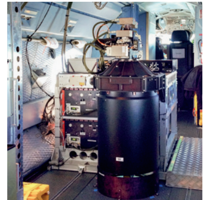
The aerosol and water vapour lidar implemented by the DLR Institute of Atmospheric Physics
