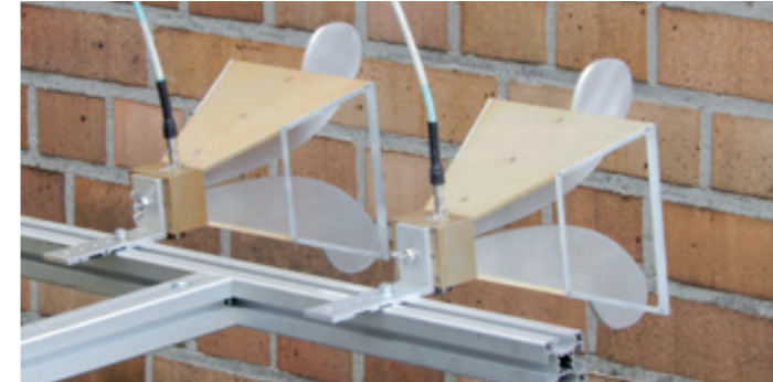
GTOM antennas examine the wall of a house
