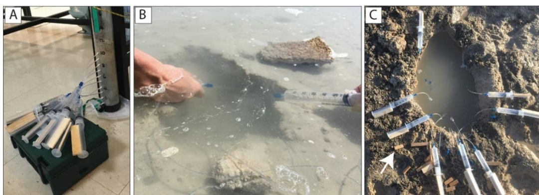
Figure 2.2. (A) ‘Traditional’ application of Rhizons into a pre-drilled core, and (B) in situ application of Rhizons, both using standard sized wooded stoppers to create a vacuum with the syringe (Oct. 2017). (C) In situ application of Rhizons using wooden stopper with sequentially increasing sizes; note the smaller stopper that had been used (arrow).
