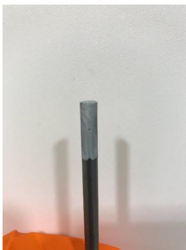
Figure 6 Zinc coated carbon electrode
