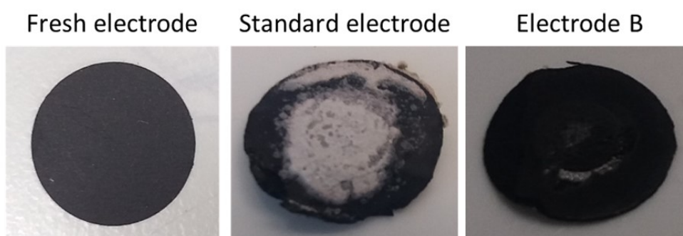
Figure A.22: Photographs of an uncycled and two cycled electrodes (126 cycles, 2 V cell voltage at dismantling) of the test cells showing silver-coloured sodium plating on the electrode surface. Electrode diameter 12 mm; Standard Electrode: 26 % porosity; Electrode B: 30 % porosity.
