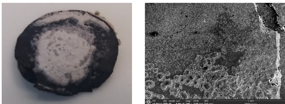
Figure A.10: Left: Photographs of cycled electrodes after disassembling showing sodium plating on the electrode surface. Electrode diameter 12 mm. Right: SEM image of the cycled electrode surface.
