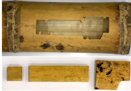
Figure 4.8. Robotically fabricated small clear bamboo samples
