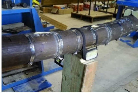
Figure 5.25. Sample eM318 showing initial outward buckling deformation in-between bands of an open reinforced section (OpenR@D).
