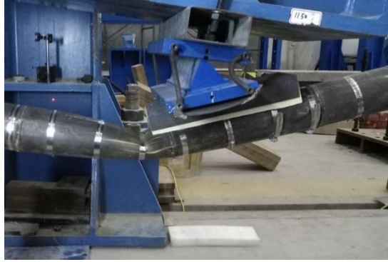
Figure 5.29. Sample eM517 displaying the typical local kink failure for closed-reinforced samples located right at the steel band and away from the loading saddle
