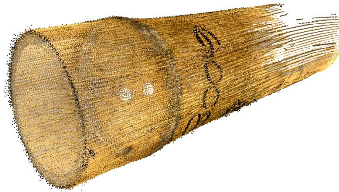
Figure 3.6. Scanned raw data of the end-section of a bamboo pole
