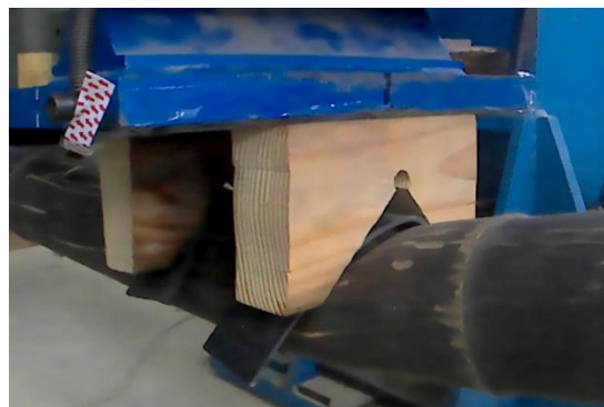
Figure 5.15. Sample eM013 loaded with short saddles, showing a combined failure dominated by local kink under loading saddle, but also developing the typical longitudinal splitting
