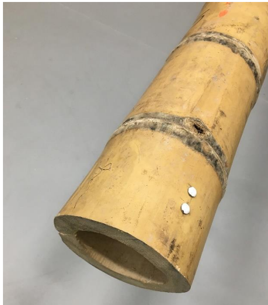
Figure 3.5. End section of bamboo pole and scanning reference markers
