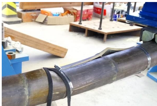
Figure 5.27. Sample eM434 showing typical outward buckling failure in-between bands of an open reinforced section (OpenR@3D)
