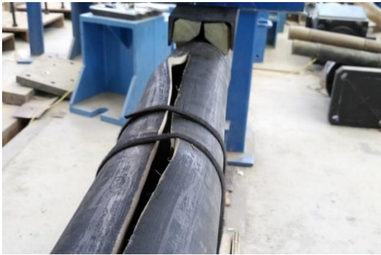
Figure 5.21. Sample eM233 showing typical outward buckling at the open ends of the cross-section. Note that the amplitude of the buckling wave at each side of the crack did not coincide.
