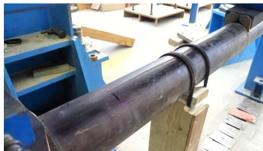
Figure 5.18. Artificial crack within the central span, a diameter away from the loading saddles and oriented towards the top of the cross-section
