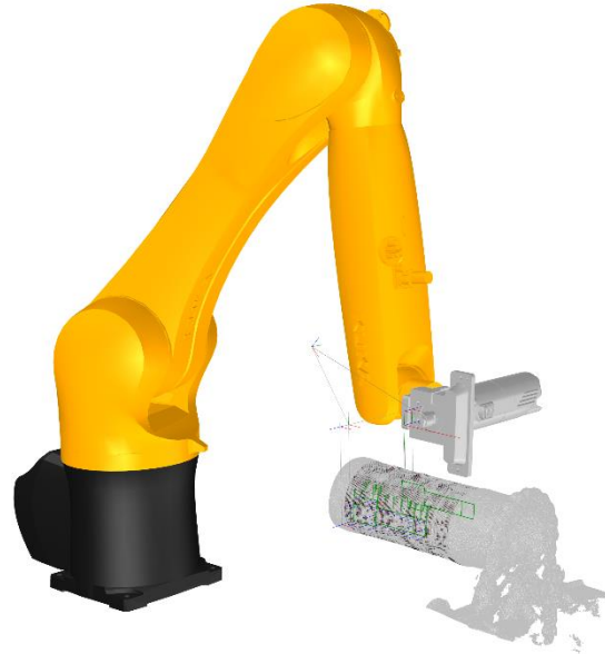
Figure 4.7. Robotic toolpath generation with KUKA|PRC [195]
