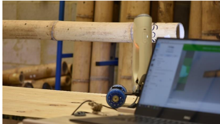
Figure 3.18. Scanning procedure on a Guadua bamboo pole
