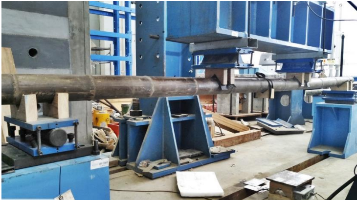
Figure 5.3. Four-point bending test
