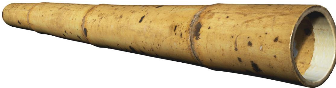
Figure 3.8. Texturized polygon-mesh model of a scanned bamboo pole
