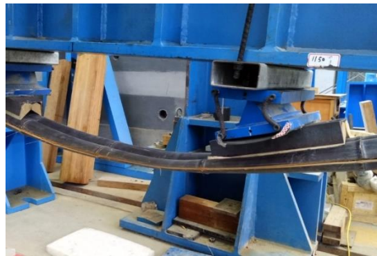
Figure 5.17. Sample eM107 loaded with single saddle displaying the typical longitudinal split failure
