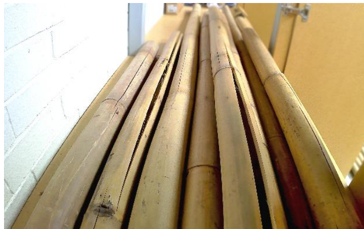
Figure 2.5. Natural splitting appearing along the height of bamboo poles
