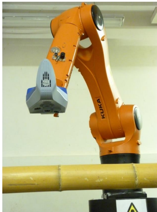
Figure 2.7. Scanning of a bamboo pole driven by a robotic arm, taken from [82]
