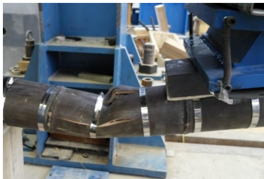
Figure 5.26. Sample eM325 displaying the typical local kink failure mechanism at the steel band, where the top of the cross-section and the band flattened out (OpenR@D).
