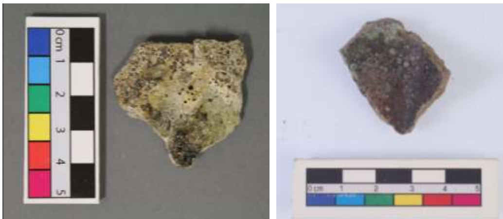
Figure 3.9. Crucible fragments with evidence of interaction between ceramic and charge. Left: A fragment from the Ashmolean laboratory (AN1999.205.31) showing intense distortion of the ceramic and a greenish discolouration due to the corrosive attack of alkalis. Right: Fragment from Jamestown (JR 2361D) with green spots on its internal surface corresponding to corroded brass prills.
