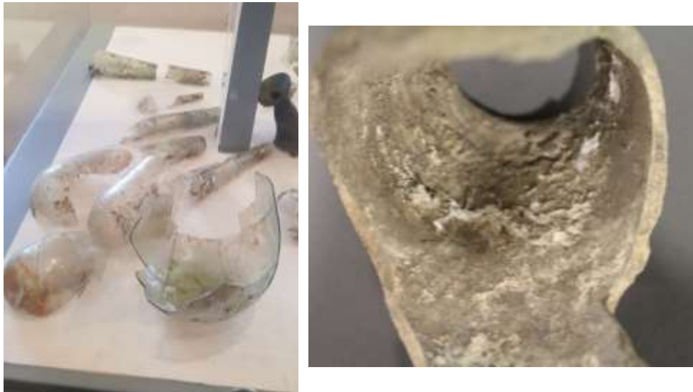
Figure 3.5. Residues left on chymical apparatus after distillation. Left: A reddish deposit can be seen on some of the glass vessels from the 16 th -century laboratory of Oberstockstall (Austria); right: one of the tall crucibles from the Ashmolean laboratory, showing a white deposit rich in zinc.
