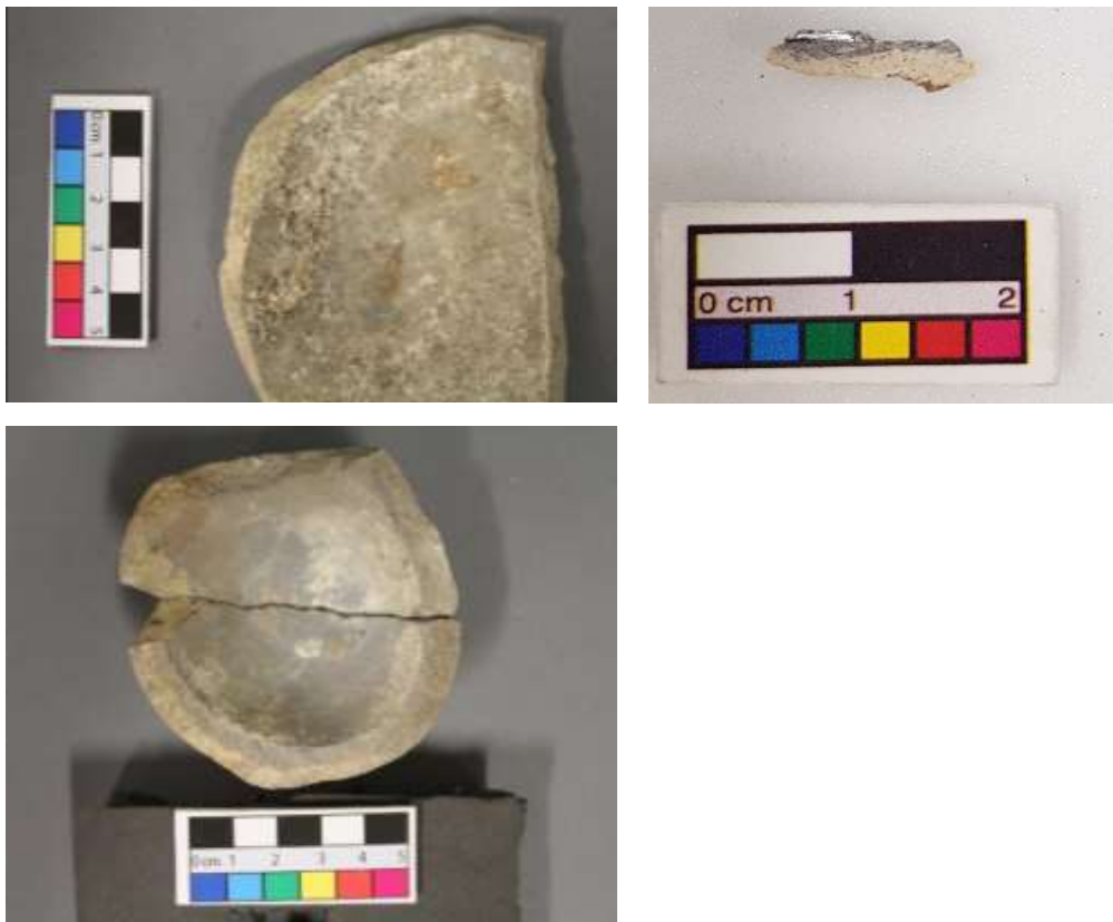
Figure 5.20. Fragments of tall crucible with closed profile used in zinc-related metallurgy. Top: Fragment of the crucible wall (left) and sample taken from it (right). Note the layer of bright metallic zinc and the dark colour of the ceramic in contact with it due to the strongly reducing conditions within the vessel. Bottom: The bottom of the same crucible showing the zinc-rich white deposit and the dark-looking ceramic resulting from the reducing atmosphere.
