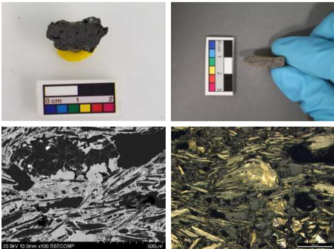
Figure 5.8. Top: Sections through the fragments of graphitic crucible AN1999.205.28 (left), analysed here, and OX1422 (right), analysed by Martinón-Torres in 2012 and belonging to a different vessel. Bottom: SEM-EDS micrograph showing the ceramic matrix of AN1999.205.28 (left). The black phases are bits of graphite, while the grey areas result strongly enriched in potash. On the right is an optical microscope micrograph of the same sample showing the flakes of graphite in yellow.
