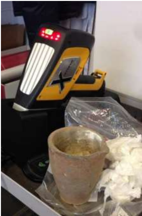
Figure 3.8. The pXRF used for the present work during the initial screening at the Ashmolean Museum (cf section 5.4).
