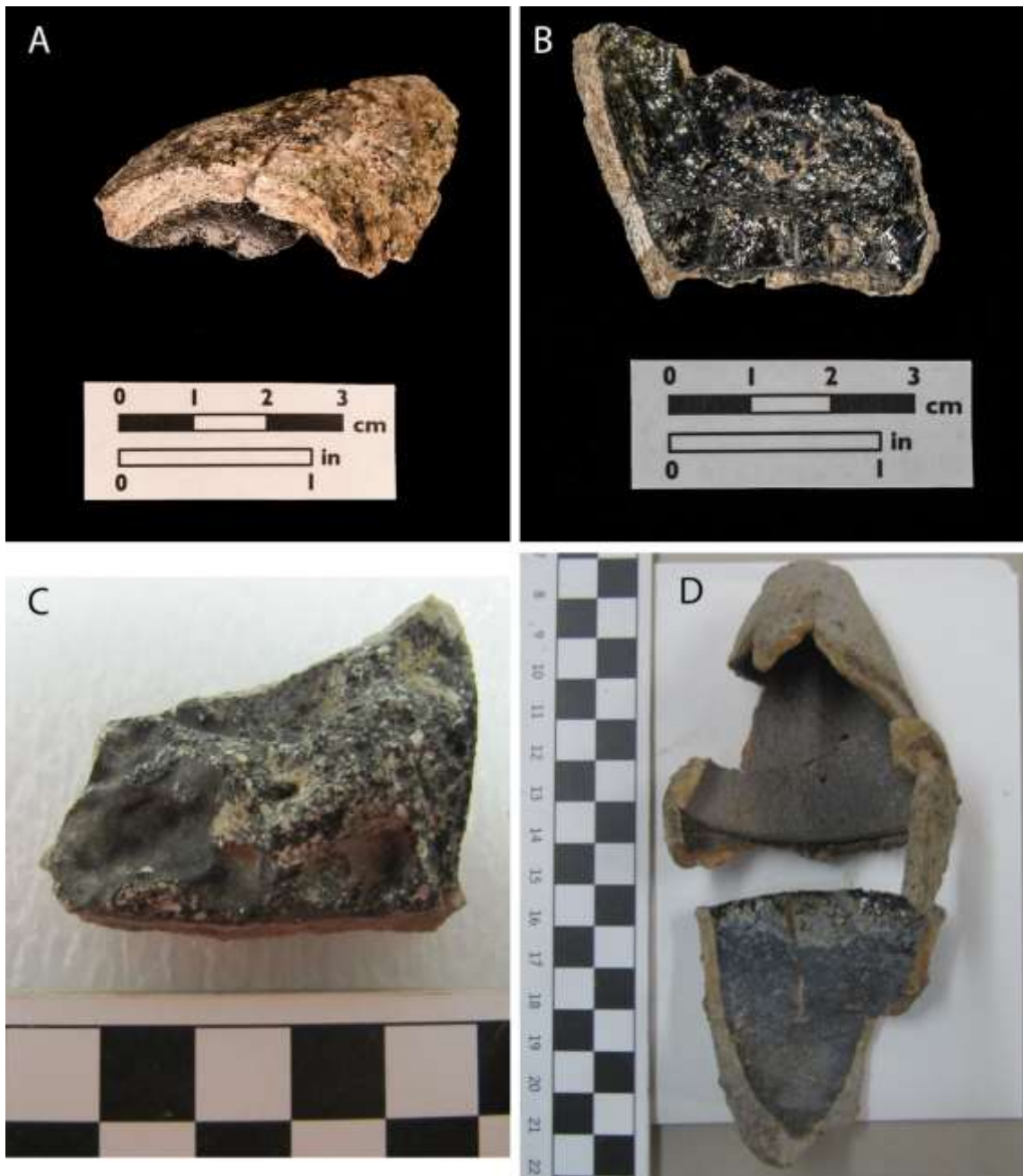
Figure 4.34 A-B: Sample J14 from Owen et al 2014. Note the smooth surface underneath the residue and corresponding to the contact area with the pool of molten metal underneath (A) and the “fin” protruding from the internal side of the vessel (B). C: Sample JR92A also showing a similar protruding feature. D: crucible fragments from the same context of JR1945C. Note the clean internal wall of the vessel, protected by the molten metal and the residue only forming towards the rim (Photos: Marcos Martín-Torres and Preservation Virginia’s Jamestown Rediscovery Foundation).
