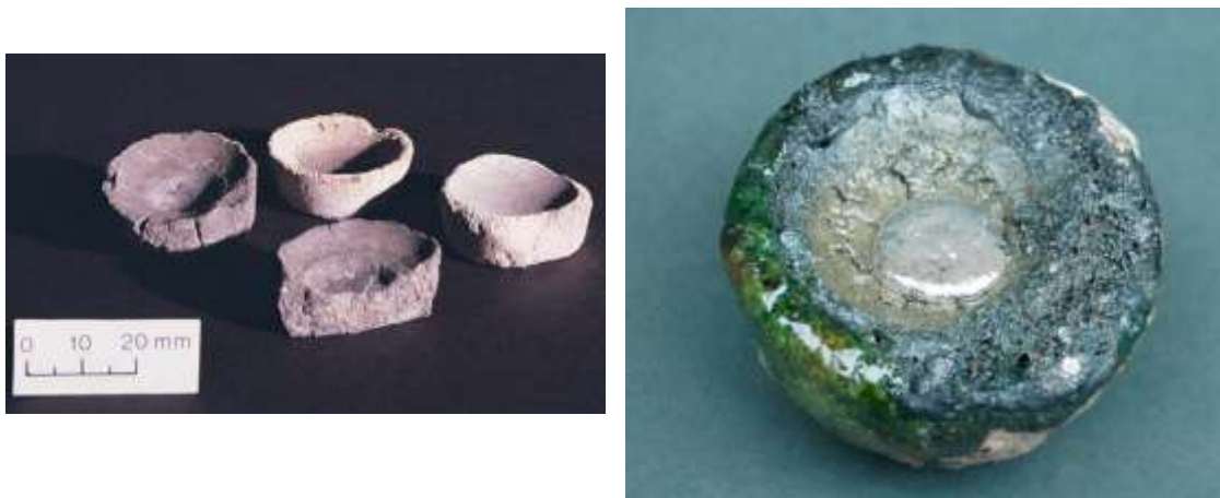
Figure 3.7. Left: A set of bone ash cupels from the Tower of London (after White 2010); right: Experimental replica of a cupel showing the silver button in the centre. Note the heavy interaction between the lead oxide and the cupel which produced the green lead silicate glaze (after Moureau and Thomas 2016).
