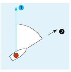
**Figure 3–1.** Difference between COG, the direction of motion with respect to the ground, ①, and Heading, the direction that a vessel is pointed at, ② (credit: Wikipedia user WolfgangW)
