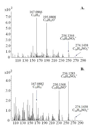
Figure 7.6. MS<sup>2</sup> spectra of (A) norhydroxydesomorphine isomer 1 and (B) norhydroxydesomorphine isomer 2. Data acquired in full scan.
