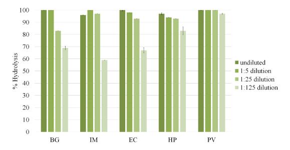
Figure 4.3. Extent of hydrolysis for IMCSzyme<sup>TM</sup> (IM), BGTurbo<sup>TM</sup> (BG), *E. coli* (EC), *H. pomatia* (HP) and *P. vulgata* (PV) at undiluted, 1:5 diluted, 1:25 diluted and 1:125 diluted enzyme levels. Error bars represent the standard deviation (n=2).
