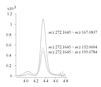
Figure 7.2. Extracted ion chromatogram of desomorphine in urine at the LOQ (0.5  $\,$  ng/mL). Table 7.5
