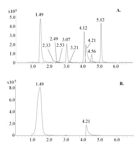
Figure 7.5. Extracted ion chromatograms for phase I metabolites (A): nordesomorphine, 4.12 min (m/z 258); desomorphine-N-oxide, 5.12 min, and hydroxydesomorphine, 1.49, 2.33, 2.53, 3.07 and 4.56 min (m/z 288); norhydroxydesomorphine, 2.49 and 3.21 min (m/z 274), and the phase II metabolite (B) desomorphine-glucuronide, 1.49 min (m/z 448). Desomorphine-D<sub>3</sub> (4.21 min, m/z 275) is shown for comparison.
