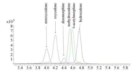
Figure 6.3. Extracted ion chromatogram depicting desomorphine (m/z 272) and closely eluting opioids (noroxycodone, m/z 302; oxycodone, m/z 316; norhydrocodone, m/z 286; 6-acetylmorphine, m/z 328; hydrocodone, m/z 300) at a 10-fold excess concentration (relative to desomorphine). Data was acquired in full scan in order to identify the elution order.
