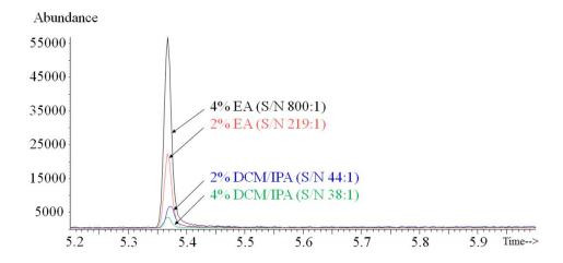
Figure 5.4. Representative EICs (*m/z* 271) of desomorphine from urine using different elution solvents. The average signal-to-noise (S/N) for each solvent (n=3) is shown in parentheses. Elution solvents: 2% ammonium hydroxide in 80:20 dichloromethane/isopropanol (2% DCM/IPA), 4% ammonium hydroxide in 80:20 dichloromethane/isopropanol (4% DCM/IPA), 2% ammonium hydroxide in ethyl acetate (2% EA) and 4% ammonium hydroxide in ethyl acetate (4% EA).
