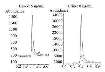
Figure 5.5. EICs of desomorphine in blood (left) and urine (right) at the limit of quantitation.
