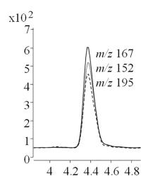
Figure 6.2. Extracted ion chromatograms of desomorphine in urine at the LOQ (0.5 ng/mL).
