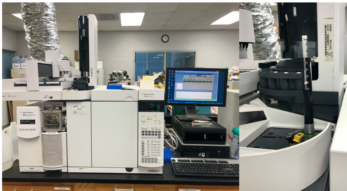
Figure 40. Full GC-MS Setup (Left) and SPME after Fiber Injection in the Inlet Port (Right).
