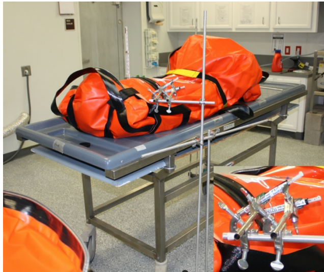
Figure 42. Zipper SPME Fiber Position. Inset shows expanded view of fiber positioning for clarity.
