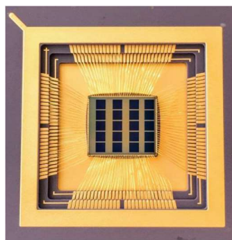
Figure 1. 20 × 1Mjot QIS test chip.
