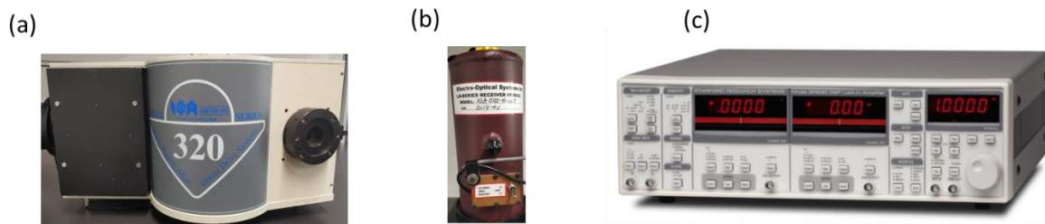
Figure 2.2.3 (a) TRIAX 322 monochromator. (b) IGA-020-E-LN7 infrared light detector mounted in LN7 Downview Dewar. (c) SR830 DSP lock-in amplifier.
