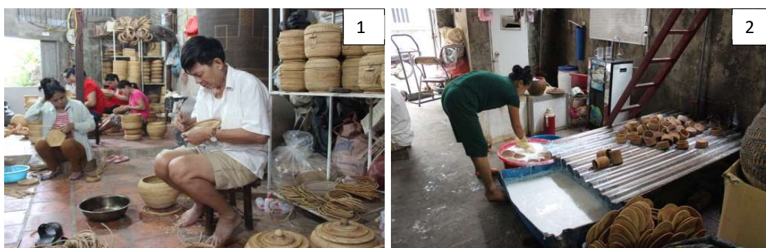
Figure 5-13. 1: Quality control section; 2: Dipping glue section
