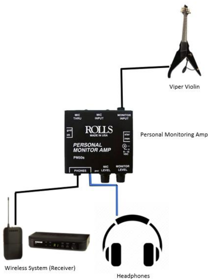
Figure 1.9. Wireless Pack Setup (Amplifier Image from Rolls Website, Violin Image from Wood Violins Website, Wireless Receiver Image from Sweetwater Website)
