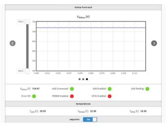
Figure 8: Voltage of the dc bus of the generator connected inverter showing some ripple
