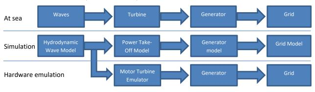
Figure 1: Sea testing Versus Simulation Versus Hardware emulation
