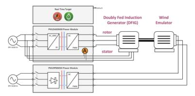
Figure 7: Wind turbine emulator lab setup
