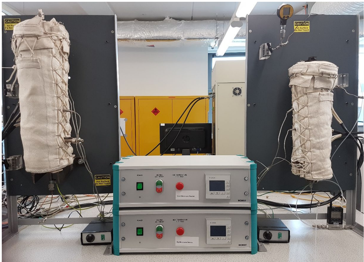
Figure 3: Photograph of the Two Membrane Reactors Enclosed in the Heating Furnace (Heating Jacket) with Power Controllers between the Reactors and Showing the Thermocouples
