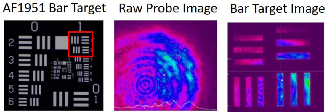
Figure 16. The raw probe image is approximately 5 mm in diameter nearly filling the CCD. The bar target is placed in the beam at the object plane of the 4f imaging system. The CCD focal plane is then placed in the image plane where the Group 1 bars are in focus. The red box illustrates the approximate field of view.
