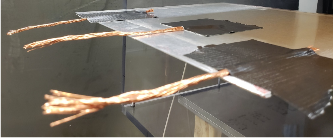
Figure 17. Airfoil with three copper wicks attached to the tapered edge with an inter-wick spacing of 7.62 cm. All wicks extend 7.62 cm past the edge.
