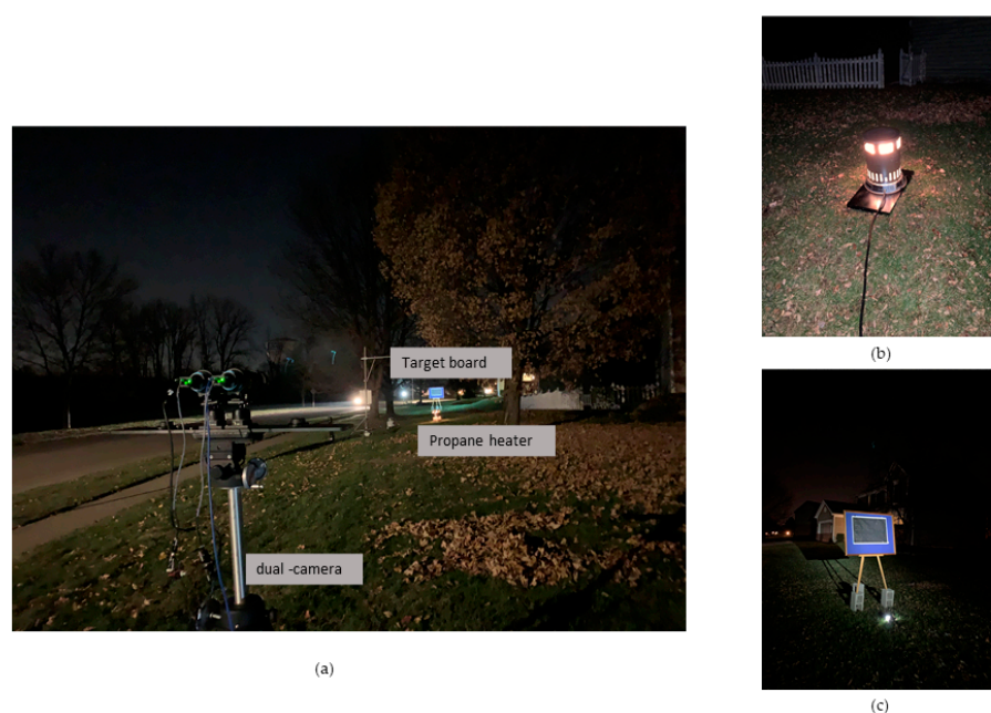
Figure 6. Experimental setup for the short-range experiment. (a) Experimental path; (b) The gas heater used to create a local spike in turbulence; (c) Target board.
