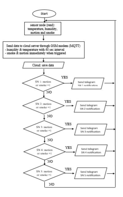
Fig. 7 - The overall flow chart of the prototype kit process
