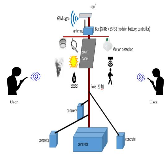
Fig. 1 - Sensor node-gateway installation
