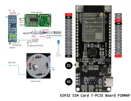
Fig. 4 - Wiring diagram for the sensor node –gateway
