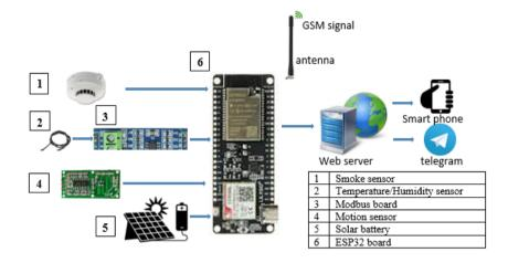
Fig. 3 - Proposed prototype kit for fire detection system
