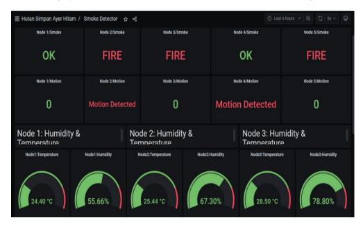
Fig. 10 - GUI for the prototype kit using Grafana software
