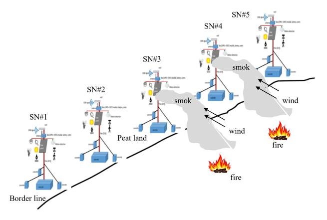
Fig. 2 - Illustration of the sensor node-gateway detects the smoke
