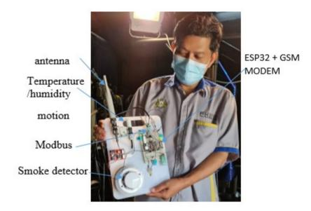
Fig. 5 - Proposed prototype kit
