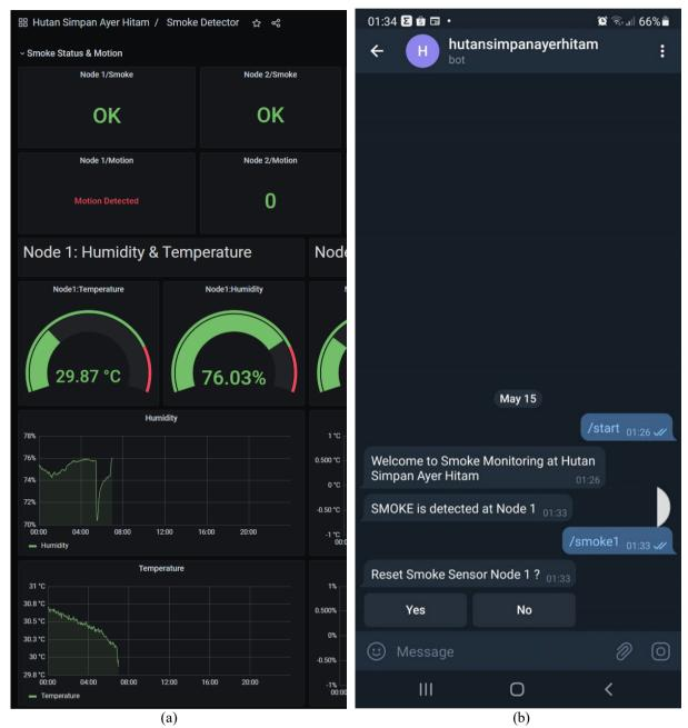
Fig. 13 - (a) GUI display using Grafana software; (b) message display in Telegram applications
