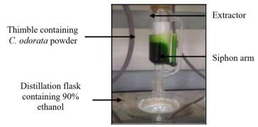
Fig. 2 - A diagram for Soxhlet extraction technique carried out in this study
