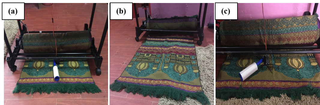
Fig. 11 - (a) Prayer mat rolls out from the platform; (b) prayer mat rolls into the platform; (c) brush turns from left to the right
