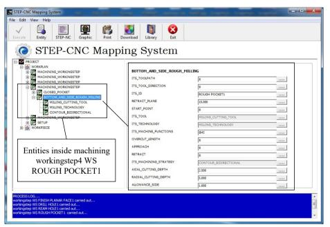
Fig. 7 - Interface for bottom and side rough milling
