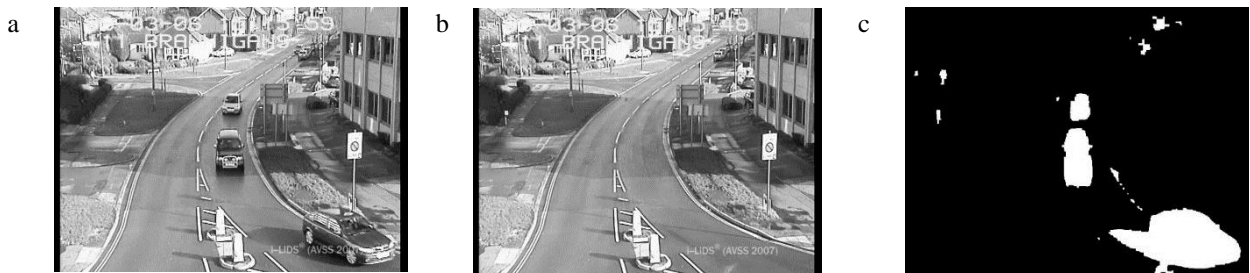
Fig. 2 - Detection and Tracking Stages for Easy Sequence from i-LIDS Dataset; (a) Current Frame, (b) Background Estimation and (c) Foreground Mask
