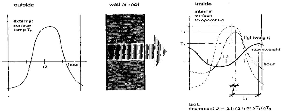
**Fig. 4 - Time lag and decrement for heavy and light constructions**
