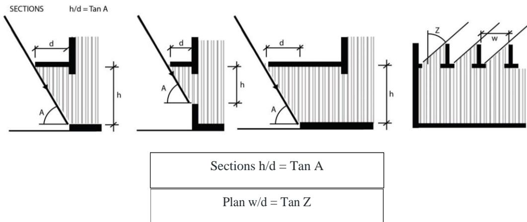
**Fig. 8 - The Geometry of shading by overhangs**
