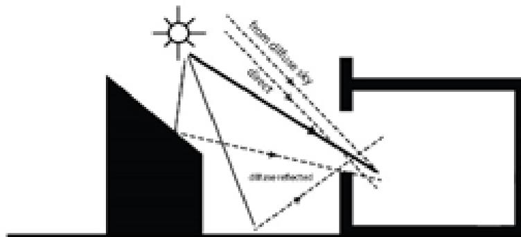
**Fig. 10 – Components of light entering a room**
