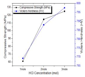
Fig. 1 Variation of compressive strength and Vickers hardness versus HCl concentration.
