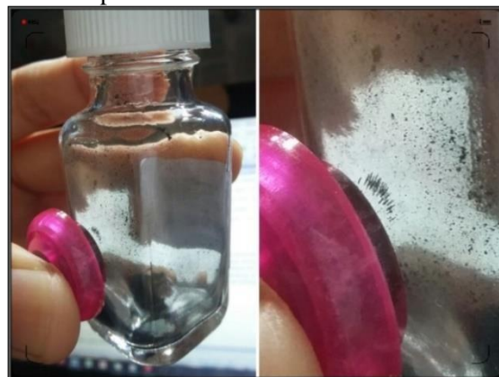
Fig. 2 Formation of magnetic field due to interactions of permanent magnet and PANI/Fe 3 O 4 hybrid nanocomposites powder.
