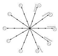
Figure 7: Output line-to-neutral voltage vector configurations (large vectors)
