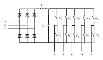
Figure 1: Five-phase voltage source inverter
