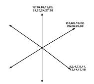
Figure 8: Input line current vector configurations (large vectors)
