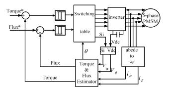
Figure 5: DTC of five-phase PMSM using standard VSI
