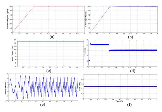
**Figure14**: Simulation of classical DTC, (a) command speed, (b) actual speed, (c) load torque, (d) electromagnetic torque, (e) stator current (phase-a), (f) stator flux
