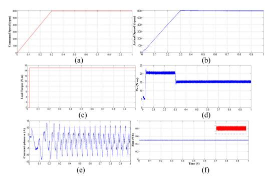
**Figure 15:** Simulation of proposed DTC, (a) command speed, (b) actual speed, (c) load torque, (d) electromagnetic torque, (e) stator current (phase-a), (f) stator flux
