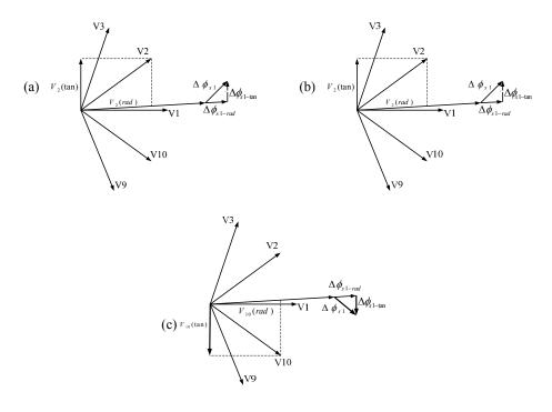
**Figure 4**: Effects of voltage vectors on electromagnetic torque and stator flux magnitude. (a) Effects of voltage vector V2, (b) Effects of voltage vector V3, (c) Effects of voltage vector V10
