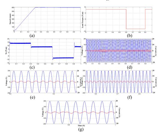
**Figure 17**: Simulation of proposed DTC, (a) actual speed, (b) load torque, (c) electromagnetic torque, (d) filtered input line current and its corresponding voltage (phase-a), (e) filtered input line current from Sec. 0.4 to 0.55, (f) filtered input line current from Sec. 0.85 to 1
