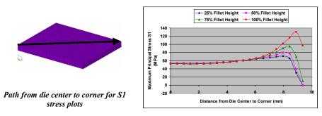
Figure 9: Tensile stress variations with different fillet height (1.61mm fillet width)
