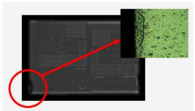
Figure 2 : Die edge crack detected in package after 500 times thermal cycling test
