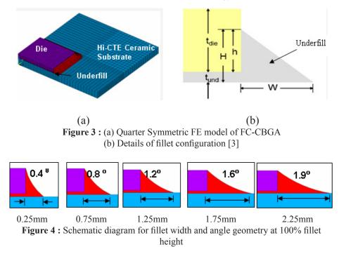
Three different combinations of CTE and Young's modulus also were used to observe the effect of material properties against thermal stress distribution. 100% fillet height and 1.61mm fillet width was assumed for all materials.
