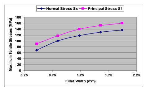
Figure 10 : Maximum tensile stress with different fillet width (100% Fillet Height)
