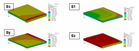
Figure 5 : Die stress distribution for fillet height 100%
