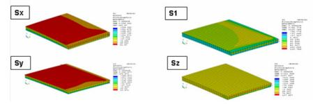
Figure 7 : Die stress distribution for fillet height 50%
