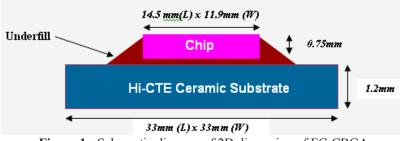
Figure 1 : Schematic diagram of 2D dimension of FC-CBGA
