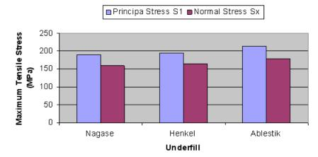
Figure 11 : Maximum tensile stress with different underfill material
