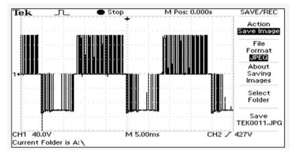
Figure 23: Voltage across resistive load at output of the prototype H-bridge circuit
