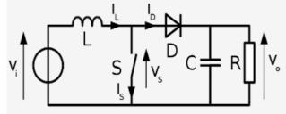
Figure 2: Boost converter schematic
