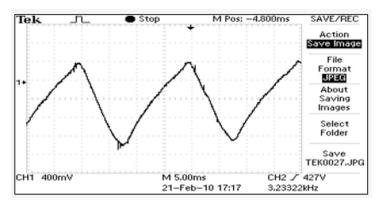
Figure 24: Voltage across resistive load after LC filtering at output of the prototype inverter circuit
