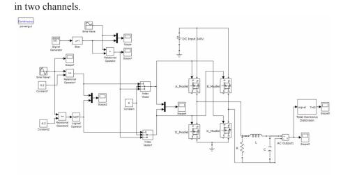
Figure 15: Simulation of designed inverter control circuit in SIMULINK
