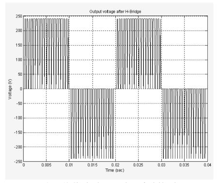
Figure 19: Simulated output voltage of H-bridge ci
