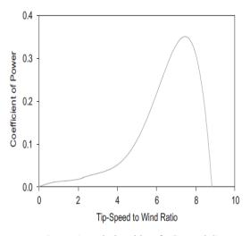
Figure 1: Relationship of TSR and C<sub>p</sub>
