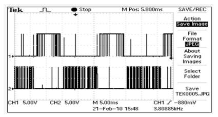
Figure 22: SPWM Trigger signals shown in two channels to the H-bridge gates
