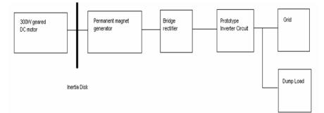
Figure 9: Proposed Lab-scale experimental rig
