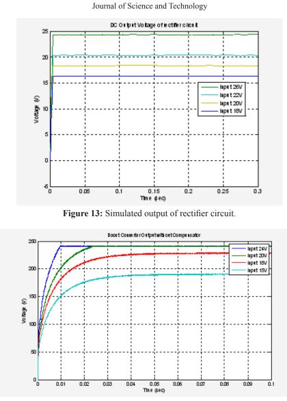
Figure 14: Simulated output of Boost DC-DC Converter
