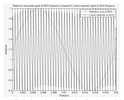
Figure 16: Simulated comparison of reference sine with carrier sawtooth signal using bipolar SPWM method in SIMULINK
