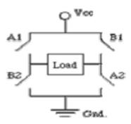
Figure 3: Standard H-Bridge circuit
