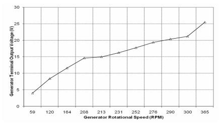
Figure 12: 500W Voltage generated at terminal of wind generator simulator rotated at different speed.
