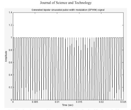
Figure 17: Simulated generated SPWM trigger signal using bipolar switching method in SIMULINK
