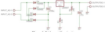
Figure 6: Bridge rectifier circuit
