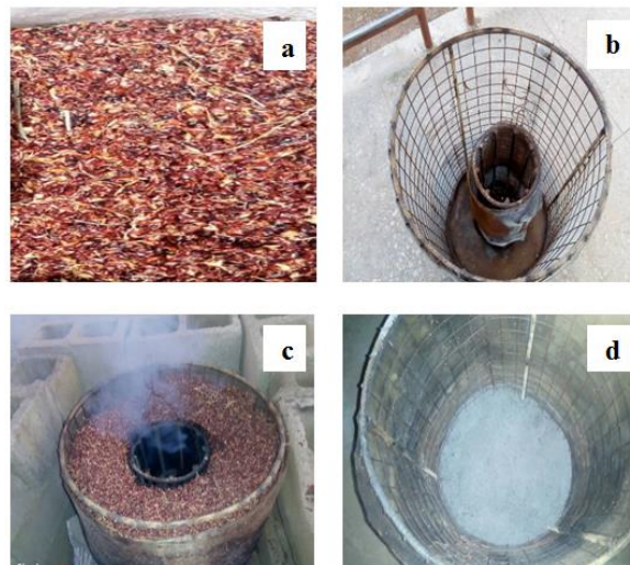
Fig. 1 - (a) sorghum husk collected; (b) set up of the locally fabricated incinerator; (c) burning into ash using the incinerator; (d) sorghum husk ash produced from the incinerator
