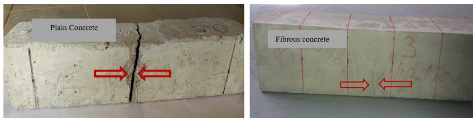
Fig. 9 - Concrete prism specimens failure pattern
