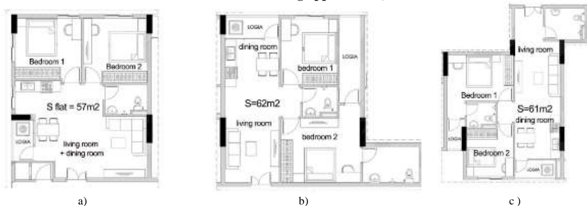
Fig. 3 - Three typical flat layouts for low-income households and worker households in Sai Dong new urban development area, Gia Lam district, Hanoi a) a two-bedroom flat, total area is 57 m 2 ; b) a two-bedroom flat, total area is 62 m 2 ; c) a two-bedroom flat, total area is 61 m 2
