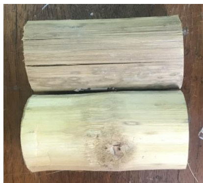
Fig. 11 - Failure pattern of compressive test specimen
