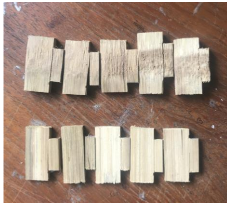
Fig. 15 - Failure pattern of shear test specimen
