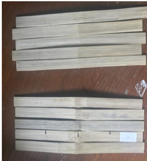
Fig. 17 - Failure pattern of bending test specimen
