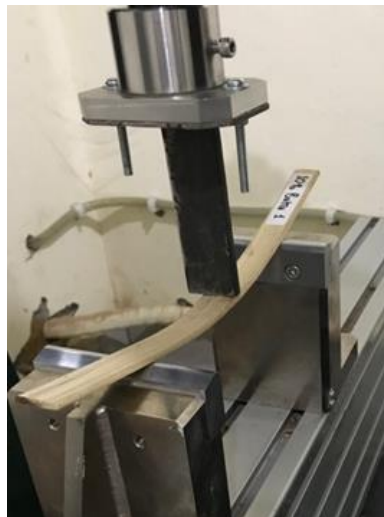
Fig. 10 - Set up for Bending Test
