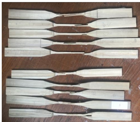
Fig. 13 - Failure pattern of compressive test specimen
