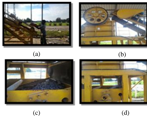
Fig. 1 - Recycle aggregates process: (a) Concrete wastes were transferred into machine; (b) Concrete wastes were transferred by conveyer; (c) Crushing process; (d) Crushed aggregates were sieved
