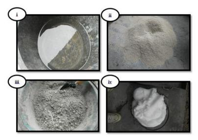
Fig. 2 - Materials of foam concrete; (i) sand, (ii) Ordinary Portland Cement (OPC), (iii) water and (iv) micro bubbles foaming
