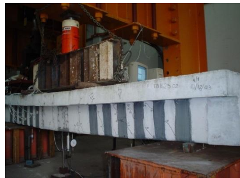
(b) CFF repaired beam -TS1-1
