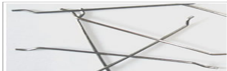
Figure 1: Hooked-end shape steel fibers used in this Study
