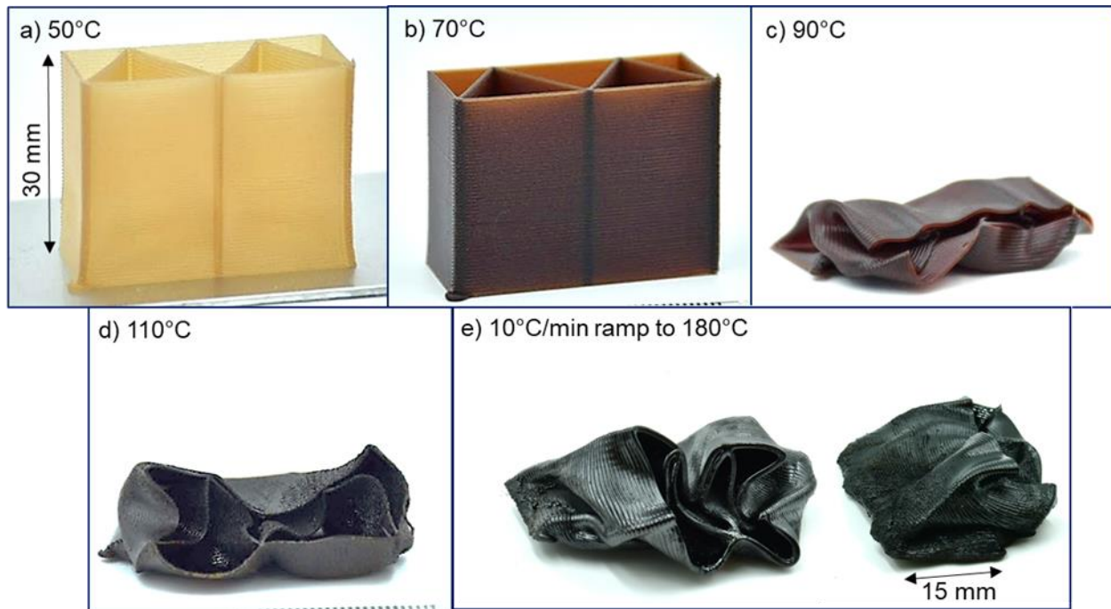
Figure 16. Single wall honeycombs printed and cured at a) 50°C, b)70°C, c) 90°C, and d) 100°C. To directly compare to the rheological temperature sweep in fig. 15, e) is cured at the same ramp rate of 10°C/min to 180°C. Prints have an average wall thickness of 0.7 mm, a height of 30 mm, and length and width of 40 and 15 mm respectively.
