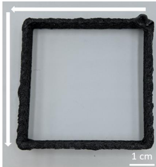
Figure 3.17: Single walled sample with rotation constant throughout the printing process
