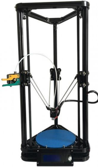
Figure 1.8: Delta 3D printer Source: [56]
