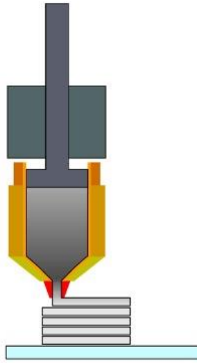
Figure 1.6: Plunger in a syringe used in direct ink writing 3D printing Source: [54]
