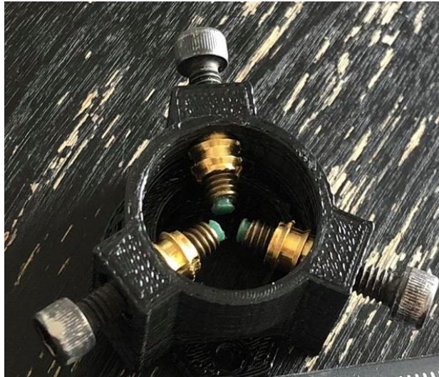
Figure 2.17: Chuck-like assembly for guiding the nozzle center to compensate for any eccentricity
