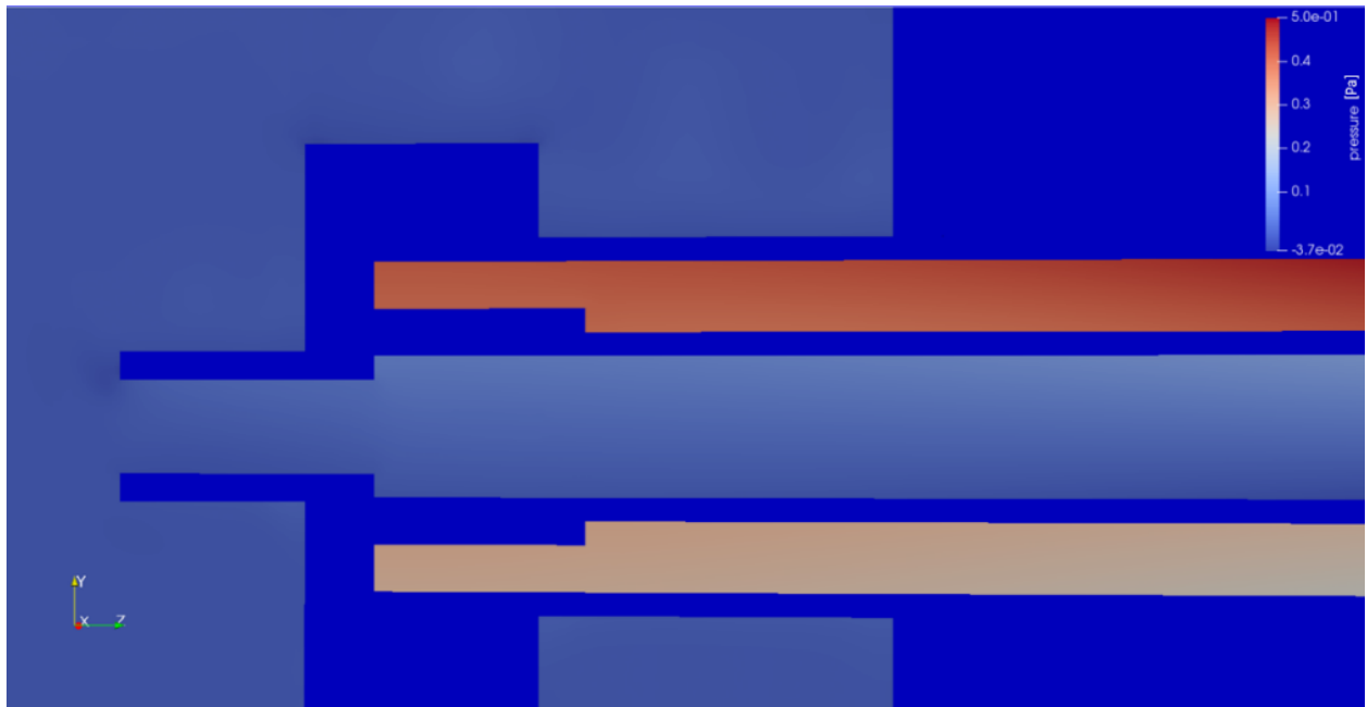
(a) Outer and inner air pressure contour plot in Pa from the 1.67 mil node mesh
