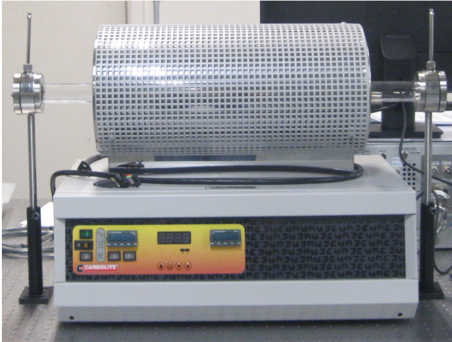
Figure 3.1: Quartz Absorption Gas Cell and Carbolite 3-Zone Tube Furnace with stainless steel flanges located at UTSI. The quartz cell sits inside the tube furnace with the steel flanges supported by posts.
